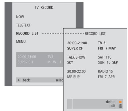
\*Overlapping recordings are indicated by OVERLAP. A red dot indicates the actual recordings which overlap. To change recording times, call up the RECORD LIST menu and edit your recordings.
