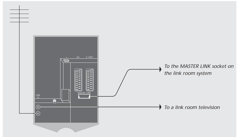
The link room system must be connected to the main room system with a Master Link cable:
