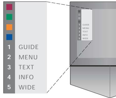
*Example of a Set-top Box Controller menu which gives you access to functions specific to your particular set-top box. – The Beo4 buttons are shown to the left on the menu and the set-top box buttons are shown to the right. Press the coloured buttons or number buttons on Beo4 to activate your choice.*
