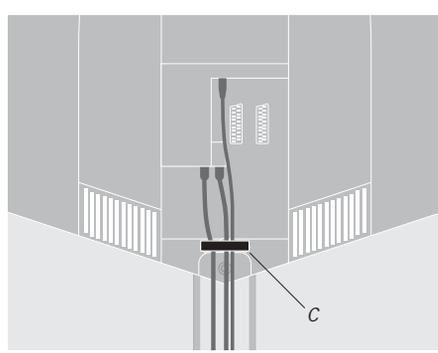
Securing the cables: For safety reasons, you must fasten all the cables running from the BeoCenter 1 with the cable band (C).
