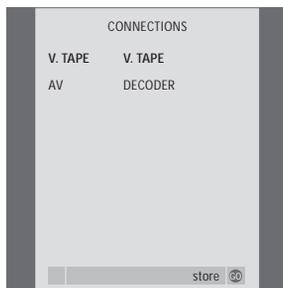
*The CONNECTIONS menu prompts you to register or confirm which type of extra equipment you have connected to the V.TAPE and AV sockets on the rear of BeoCenter 1.*
