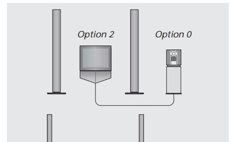
*BeoCenter 1 and an audio system set up in one room – all speakers are connected to the BeoCenter 1.*
