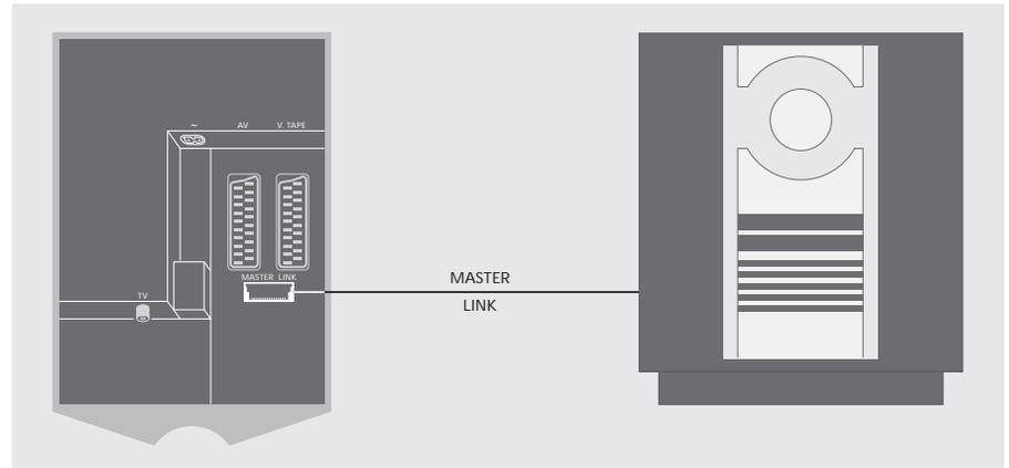
Make the connection between the BeoCenter 1 and the audio system using a Master Link cable:
